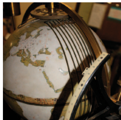
Figure 10. The declination scale and the twilight wires. (Courtesy of the National Maritime Museum, Greenwich, London.)
