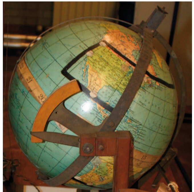
Figure 5. The Machine's declination axis scale. (Science Museum / Science & Society Picture Library)
