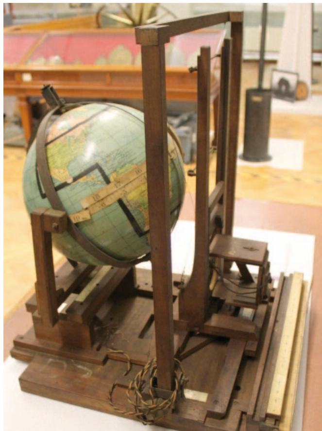
Figure 2. McNeile's wooden Occultation Machine. (Science Museum/Science & Society Picture Library)
