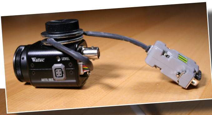
Fig.5 The camera with the replacement attached. On top the strain relief with two washers and an 1/4" screw. The D-SUB 9 has a coloured marking.
