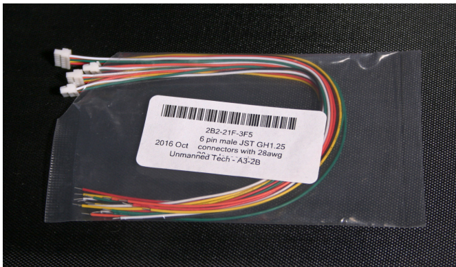
Fig.3 The package of five connectors with wires I have got from U.K. One is already in use. The wires are 20 cm long.
