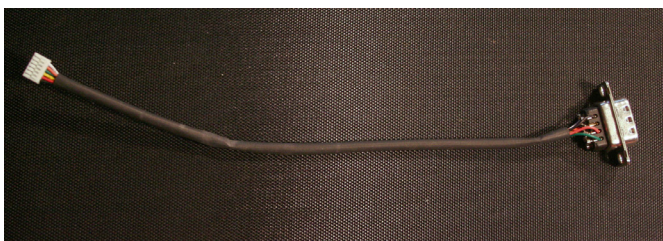
Fig.4 The male D-SUB 9 without housing is connected to the replacement cable. A piece of heat shrinkable tubing protects the small wires.
