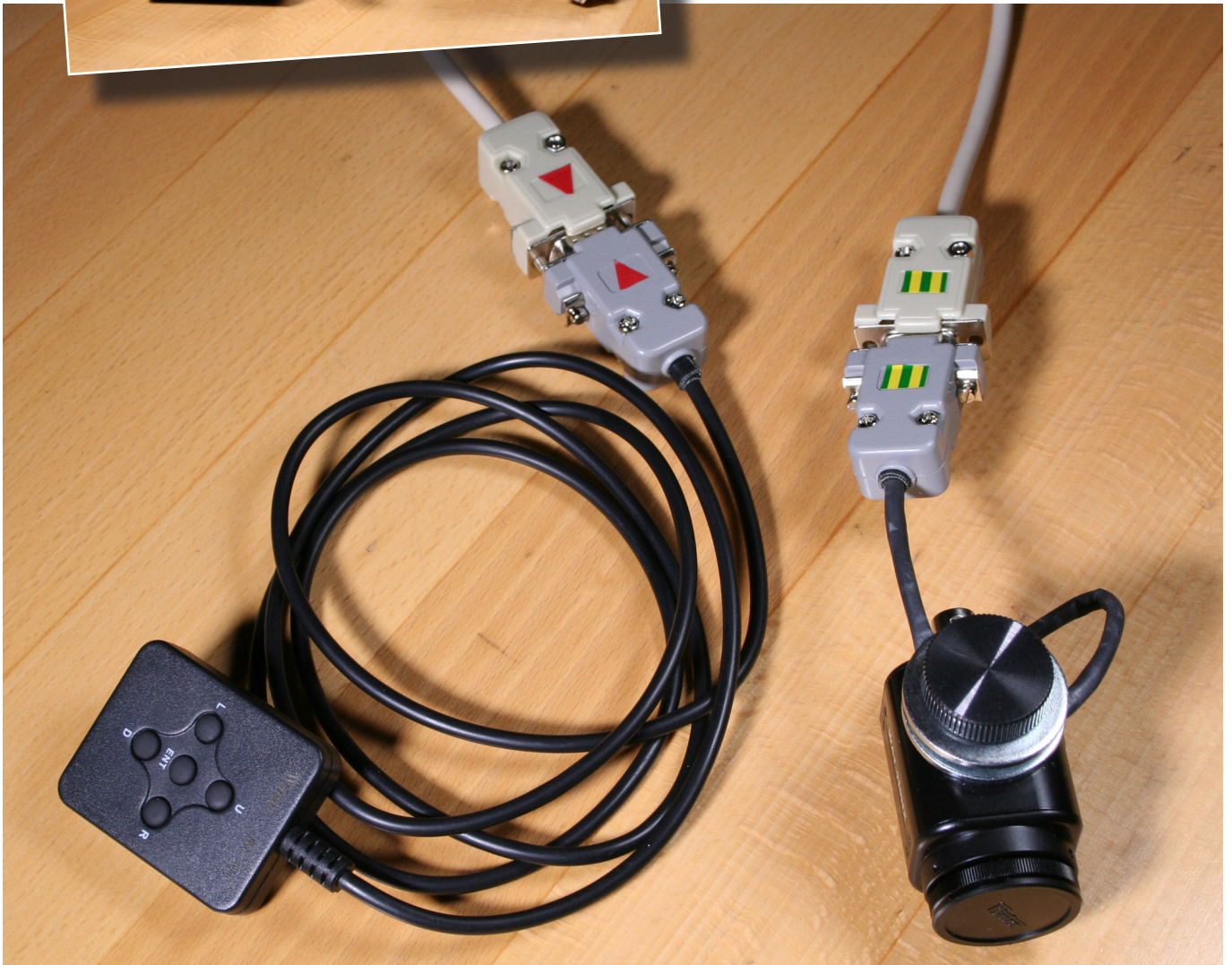
Fig.6 Camera with cable replacement, the extension D-SUB cable and the original remote cable with attached D-SUB connector. The connectors are marked for handling under bad light conditions.
