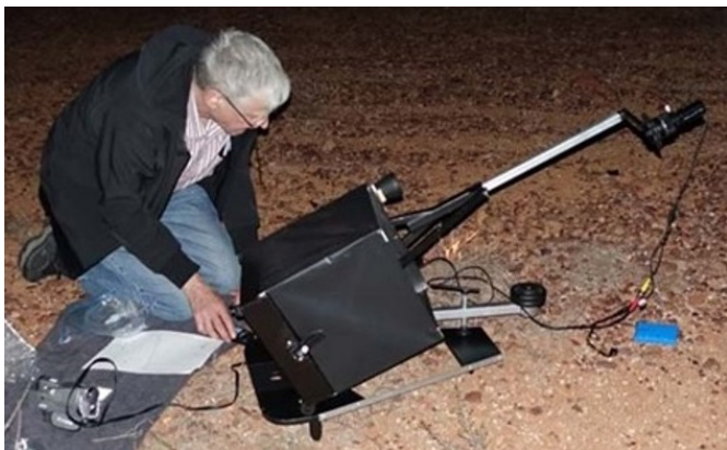
Fig. 12. A 10-inch suitcase telescope deployed in Australia, like those used at Stations 6 and 7 in North Carolina.
