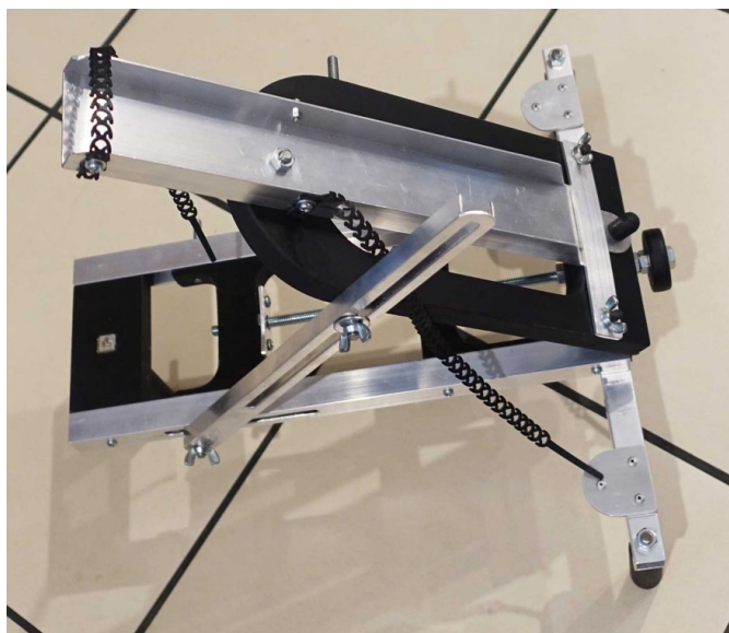
Fig. 5. John Broughton's paver mount design for an 80-mm short-tube refractor.
