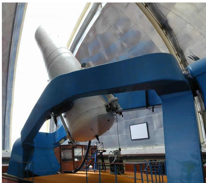
Figure 1. 1.0-m Schmidt telescope at Llano del Hato National Astronomical Observatory, Merida, Venezuela.
