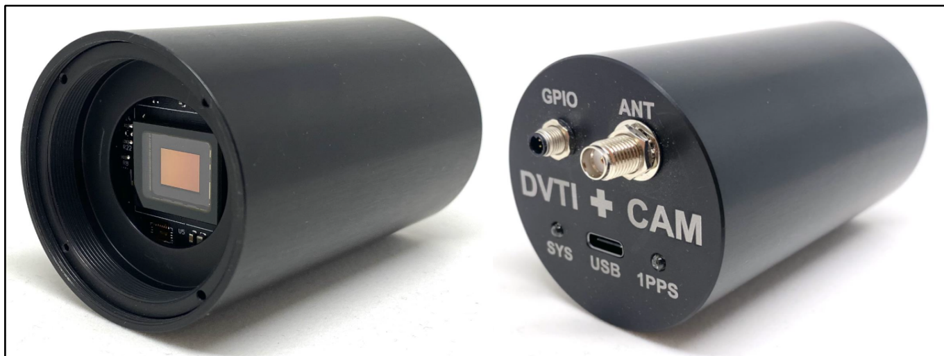
Figure 1. DVTI+CAM front view (left), with the CMOS image sensor as well as 2-inch and M42 inner threads. The rear view (right) shows the antenna connector which supports active and passive antennas for GPS, Galileo, Glonass and Baidou. The camera gets power and provides data via the USB-C connector at a maximum of 5 Gb/s.
