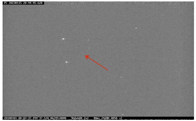
Figure 7b. Finder image, averaged from 16 individual frames recorded by the DVTI+CAM 174 in recording 2. The red arrow points to the faint star target 3 which is barely visible even in this finder image.
