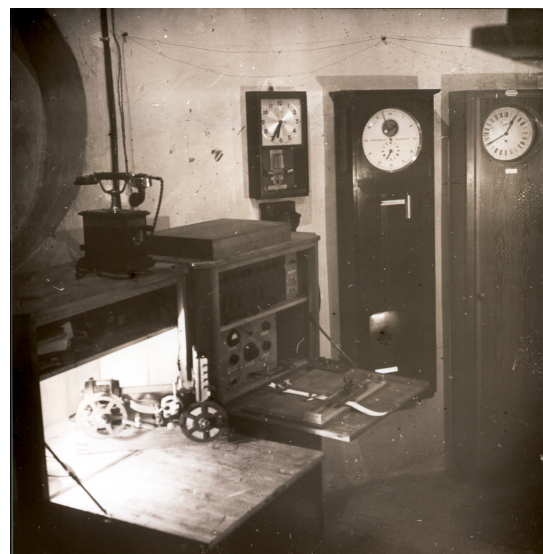
Time keeping devices at Stuttgart Observatory for the registration of occultations (approx. 1950).
